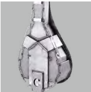
Combustion chamber (back): external air inlet and combustion air preheating.
